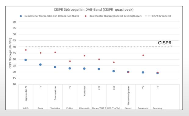
Dotted line – CISPR limit (3m, 120kHz, quasi-peak detector) Blue dots- interference level measured at 3m Red dots- interference level at actual installed distance
